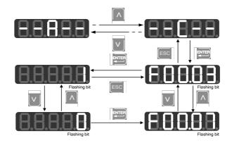
Figure 4–7 Changing Function Parameters under Non-Factory Defaults Mode
