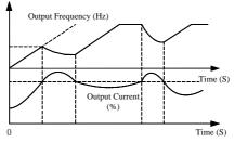
Figure 7-21 Current Limit Action Procedure
