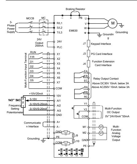
Figure 3-21 Standard Wiring of Control Circuit
