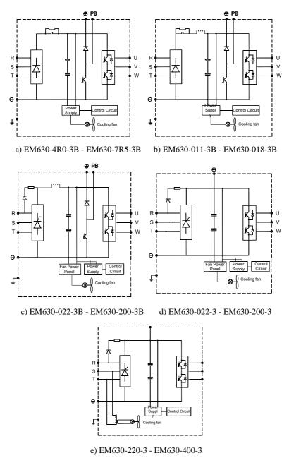
Figure 3–3 Internal Main Circuit of Inverter
