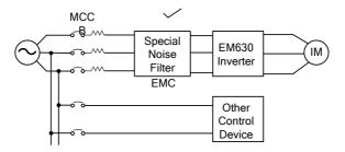
Figure 3-6 Correct Installation of Noise Filter
