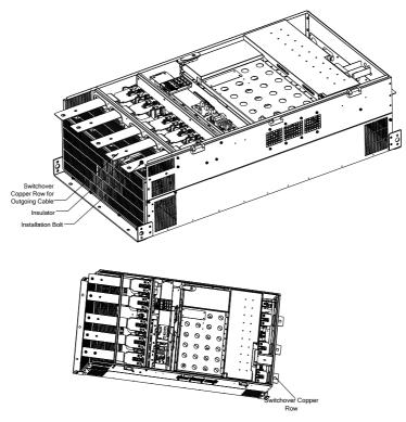
Figure 11–2 Installation of Switchover Copper Row of Outgoing Cable
