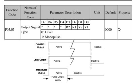
Figure 7-12 Numeric Output Terminal Level and Monopulse Output
