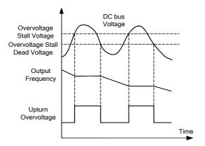
Figure 7-20 Overvoltage Stall Protection
