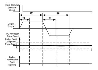
Figure 7-31 Braker Check Logic
