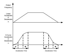
Figure 7–15 Acceleration/Deceleration Time Control
