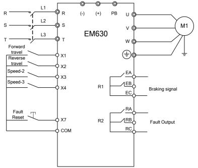
Figure 13-4 Wiring Diagram of EM630 Inverter for Travel Application of Tower Crane
