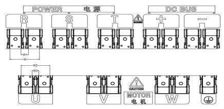
f) Main Circuit Terminal Block of Models (220-400 kW)
