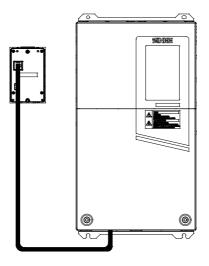
Figure 3-22 Wiring of Keypad Extension Line
