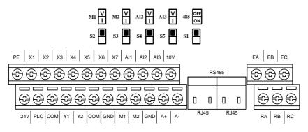
Figure 3-12 Control Circuit Terminal Block
