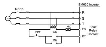
Figure 3-5 Connecting to Input Circuit Breaker
