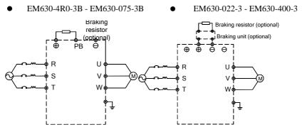
Figure 3-4 Standard Wiring of Main Circuit
