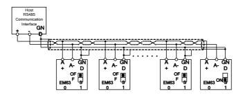
Figure 3-19 Wiring of Communication Interfaces of Multiple Inverters
