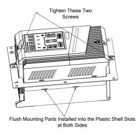
Figure 2–7 Left and Right Accessories for Flush Mounting
