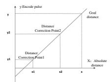
Figure 7–38 absolute distance - number of encoder pulses curve.
