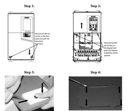
Figure 2–3 Disassemble the Keypad
