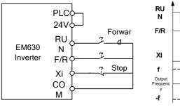
(a) F00.03=0 3-Wire Sequence Wiring Diagram
