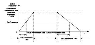
Figure 7-24 Acceleration/Deceleration Time
