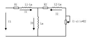
Figure 8-1 Equivalent Circuit of 3-Phase Induction Motor
