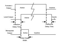
Figure 7-14 Numeric Output Terminal Level and Monopulse Output
