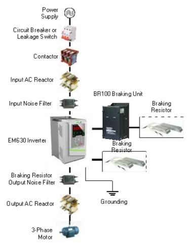
Figure 3-1 Connection of EM630 Inverter and Peripherals
