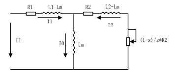
Figure 7–5 Stable Equivalent Model of Induction Motor
