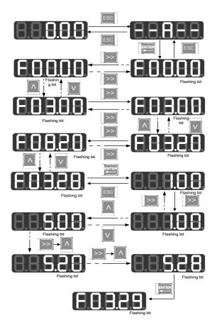
Figure 4-3 Operation Procedure from Power-on to Setting F03.28=5.28
