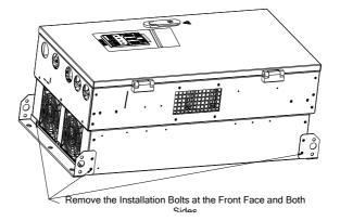
Figure 2-5 Disassemble the Top and Bottom Mounting Holes
