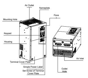
Figure 1-4 Description of Parts of EM630 Inverter (30 kW)
