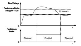
Figure 7-27 Resistance Brake
